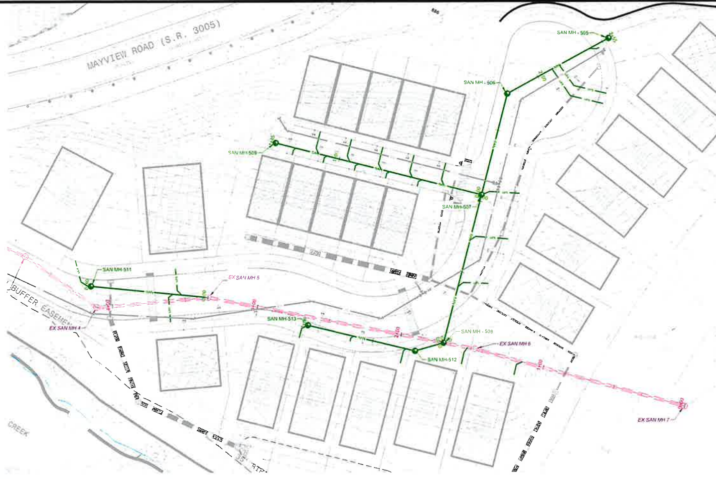
PLAN VIEW SAN MH-512 TO SAN MH-508 SAN MH-508 TO SAN MH-505 SAN MH-509 TO SAN MH-507 SAN MH-511 TO EX SAN MH
