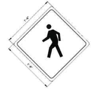
5 PEDESTRIAN CROSSING SIGN C602
